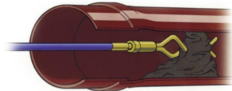
Double Worm Screw: Pierces blockages such as paper or rags and the obstruction is drawn back to clear the pipe.
